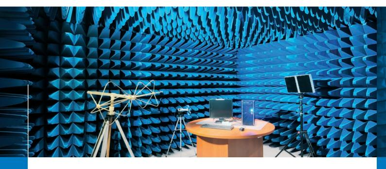
Anechoic chambers (AEC) are used in various industries to carry out scientific research and to monitor compliance with the requirements of various industry standards.
