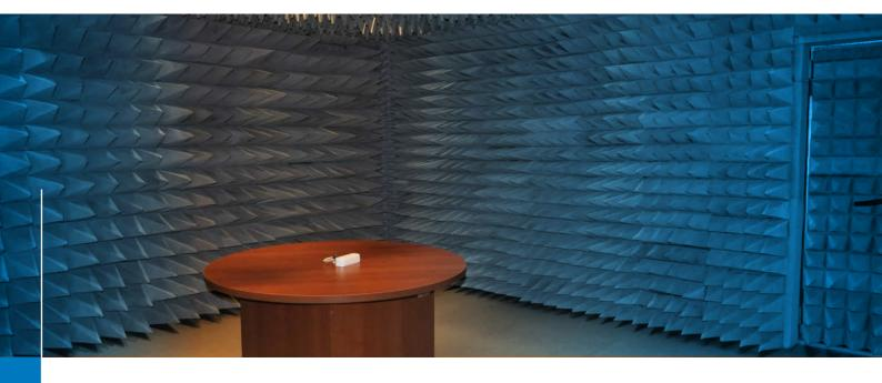
A chamber with a 3-meter measuring distance. It is a fully compliant anechoic chamber with a measuring distance of 3 m and a frequency range from 30 MHz to 40 GHz. The size of the quiet zone is  $1.5 \times 1.5 \, \text{m}$
