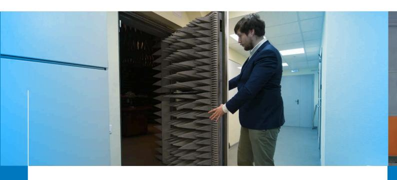
A chamber with a 10-metre measuring distance. It is a fully compliant anechoic chamber with a measuring distance of 3 m and 10 m and a frequency range from 30 MHz to 40 GHz. The size of the quiet zone is  $5 \times 5$  m.
