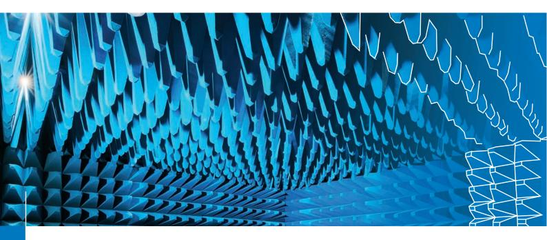
MASCOM Group supplies and installs radio-absorbent materials (RAM) of the volumetric resistive type of own production. RAM series «Eridan» is a tetrahedral pyramid made of polymer materials with ultra-dispersed carbon filler.
